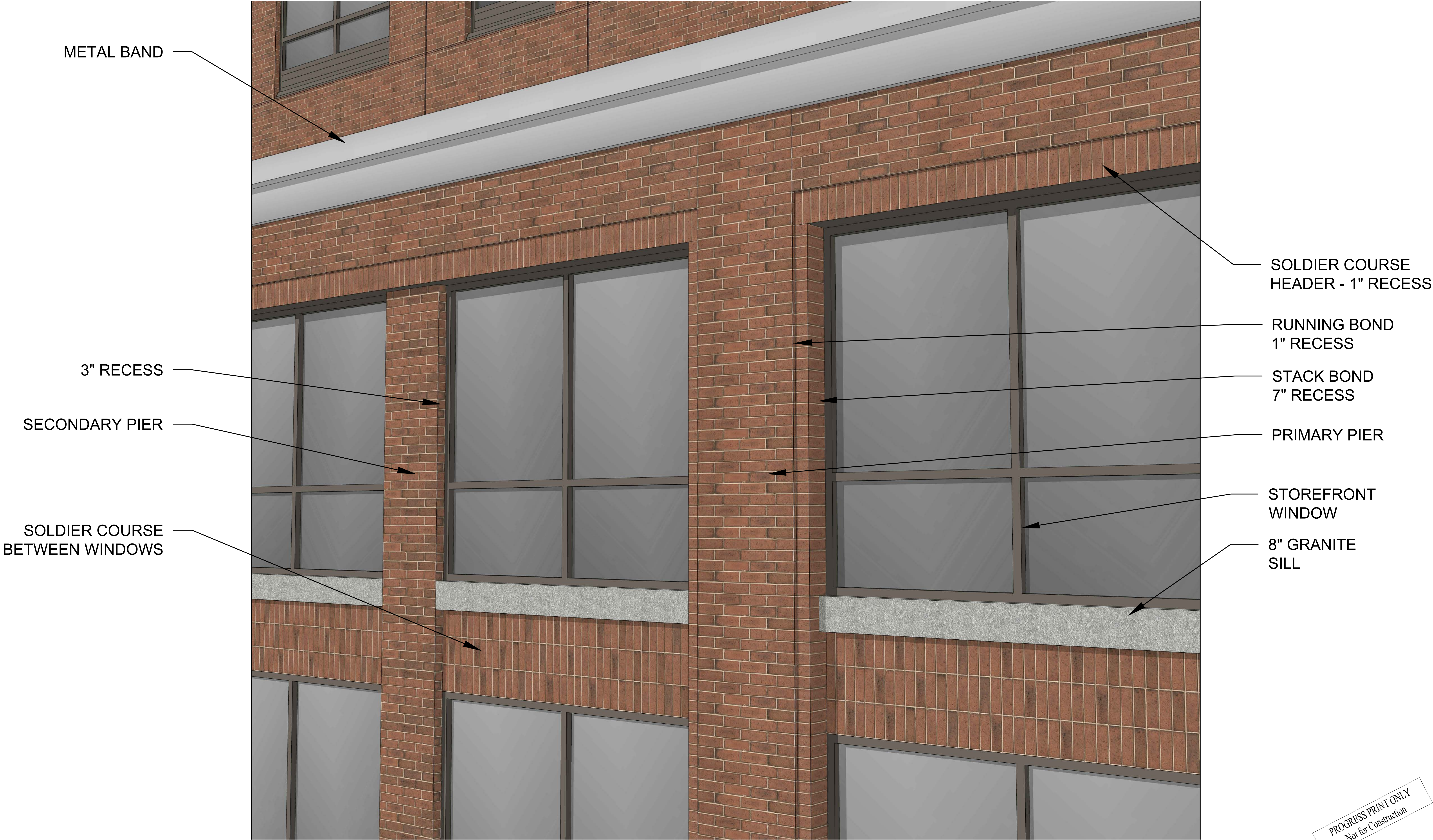
1 IMAGE DETAIL AT 3RD FLOOR STOREFRONT NTS
