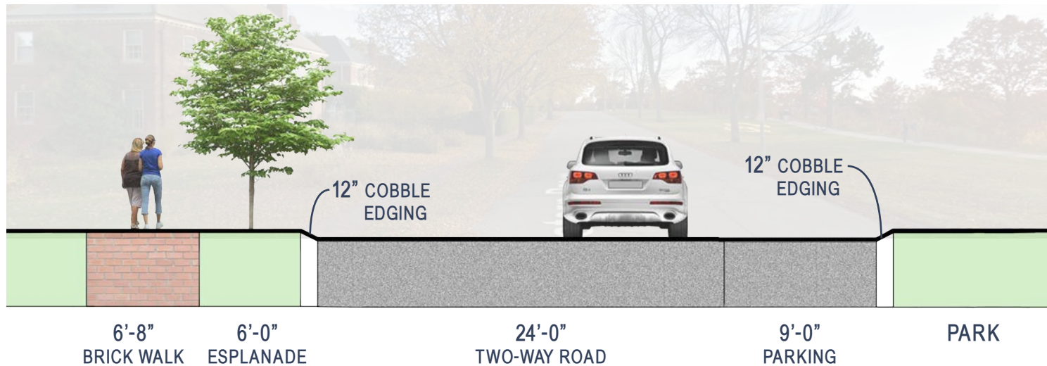
SECTION E-E': PROPOSED CONDITIONS
