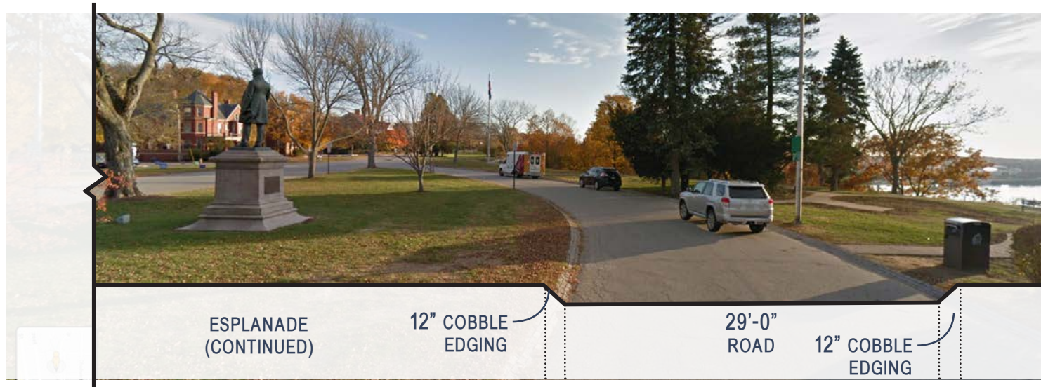
SECTION C-C': PROPOSED CONDITIONS (CONTINUED)
