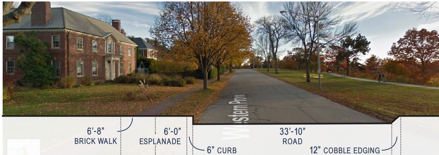
SECTION E-E': PROPOSED CONDITIONS
