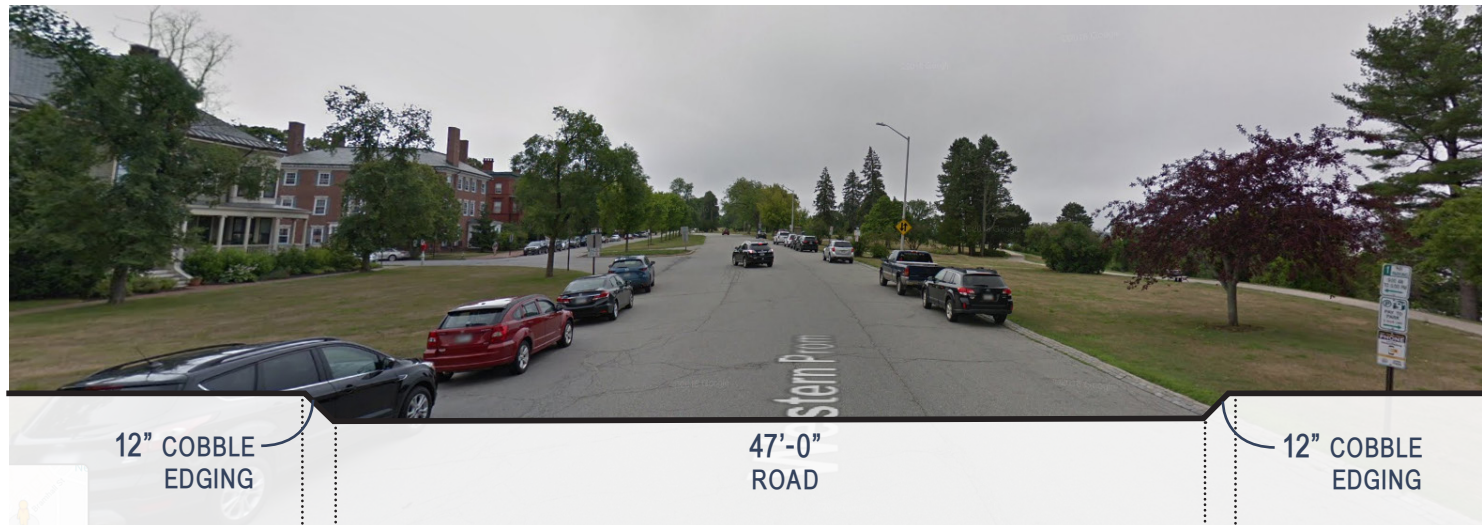
SECTION B-B': PROPOSED CONDITIONS
