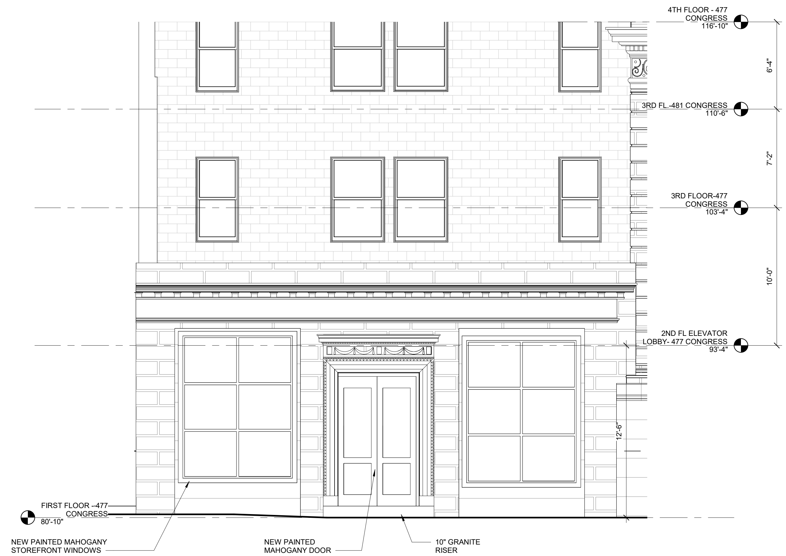
1 | CONGRESS STREET FIRST FLOOR BANK ELEVATION - NEW 1/4" = 1'-0"
