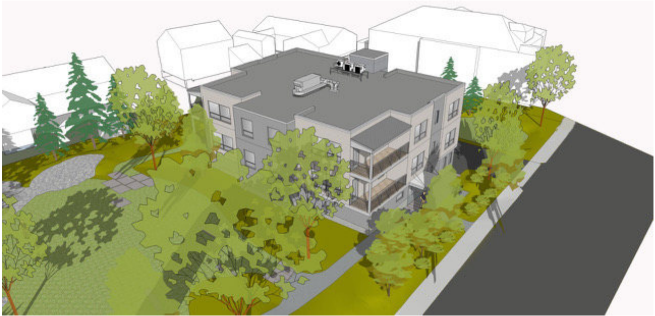
Rendering showing rooftop equipment & articulated porch roofs.
