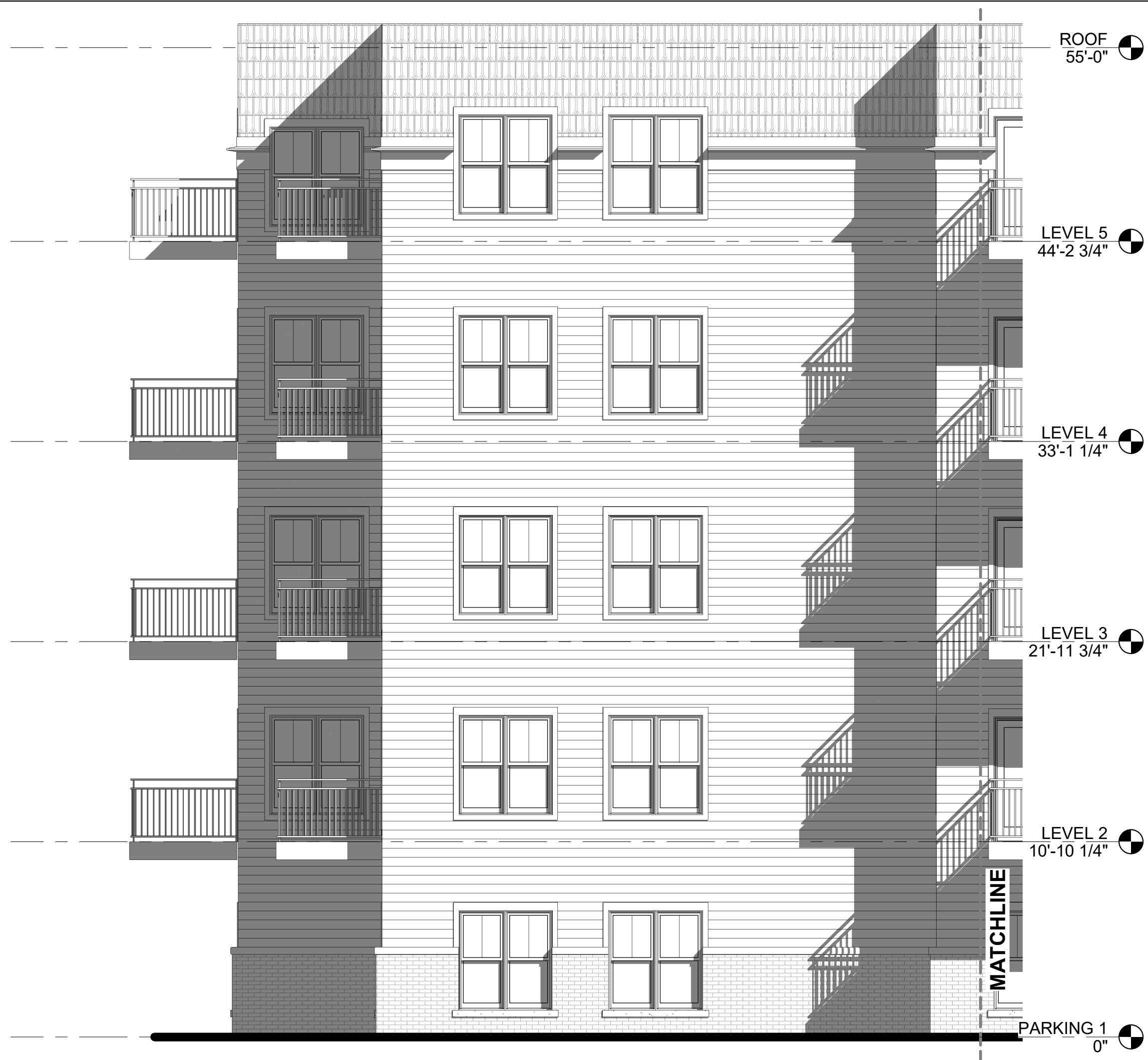
2 EAST ELEVATION - SOUTH END 3/16" = 1'-0"
