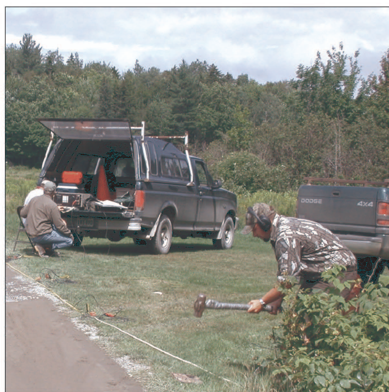
Operating a twelve-channel seismicograph, Piscataquis County, Maine.
