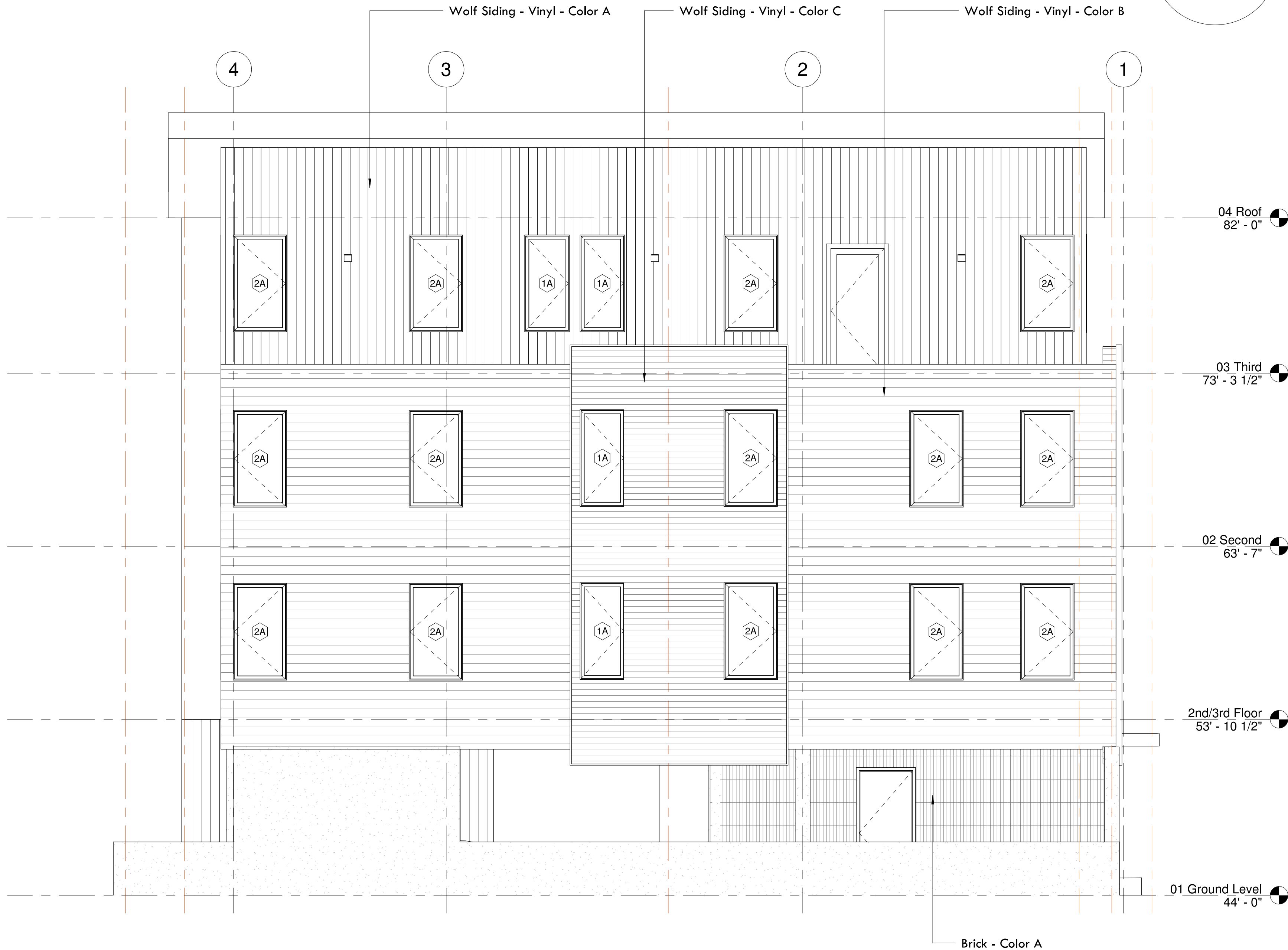
① Elevation - Cleeves Street 1/4" = 1'-0"
