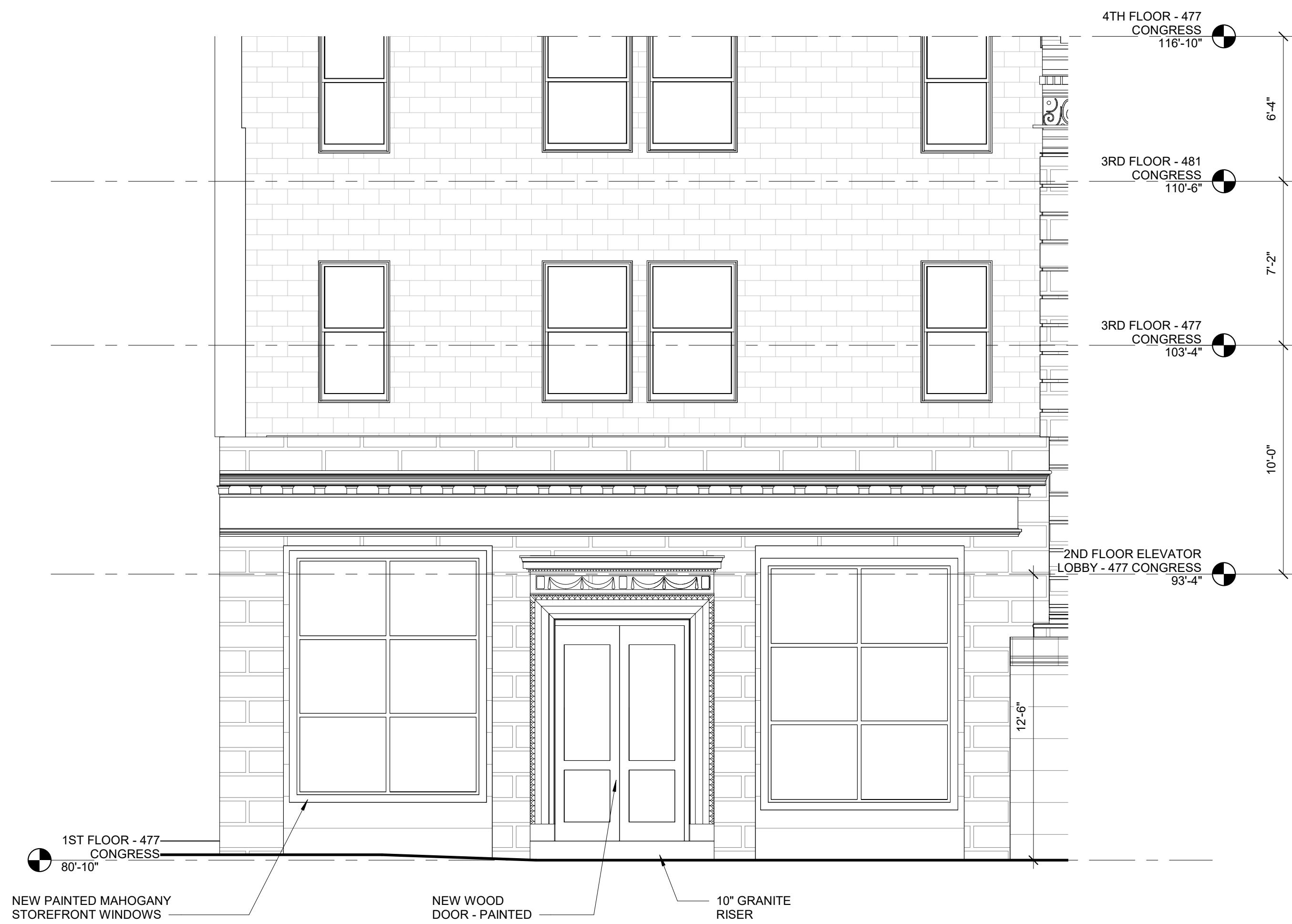
1 | CONGRESS STREET FIRST FLOOR BANK ELEVATION - NEW 1/4" = 1'-0"
