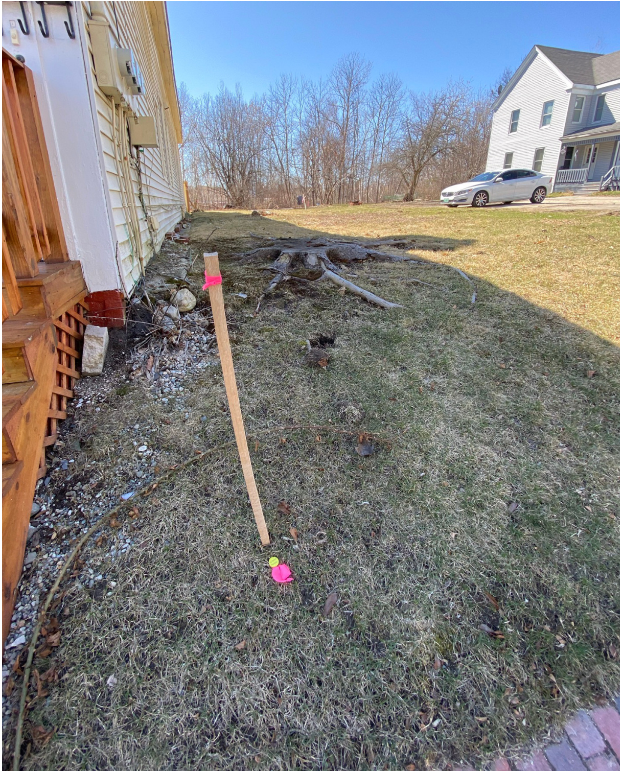
Southern parcel boundary (pin with flag) adjacent to 384 St. John Street. Shadow line is 5'-0" off pin, illustrating setback of building from lot line. Existing building on parcel, to remain is visible at right. The rear boundary of the parcel is adjacent to the tree line. Beyond lies a wide rail corridor between the active rail line and Hood Dairy's warehouses beyond.
