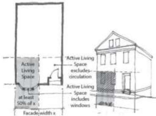
FIGURE 8-H: FRONT FAÇADE - ACTIVE LIVING SPACE
