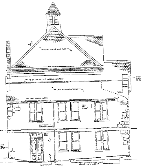
2 PROPOSED EAST EXTERIOR ELEVATION - BECKETT STREET A-13.2
