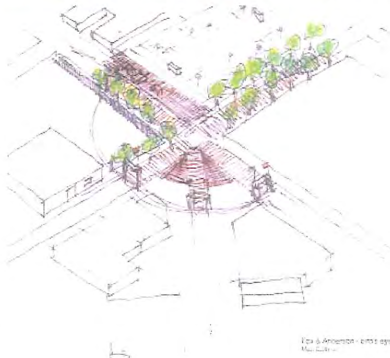
Bottom: Bird's eye sketch showing brick paving, street trees and a gateway.
