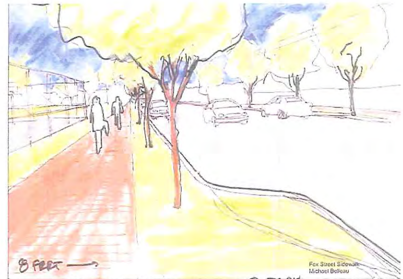
Sketch of sidewalk with curb extension, storm water parkway and trees.
