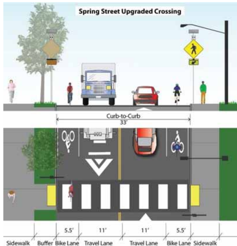
Figure 9. Upgraded Crosswalk with Rectangular Rapid Flashing Beacon on Broadway at Spring Street
