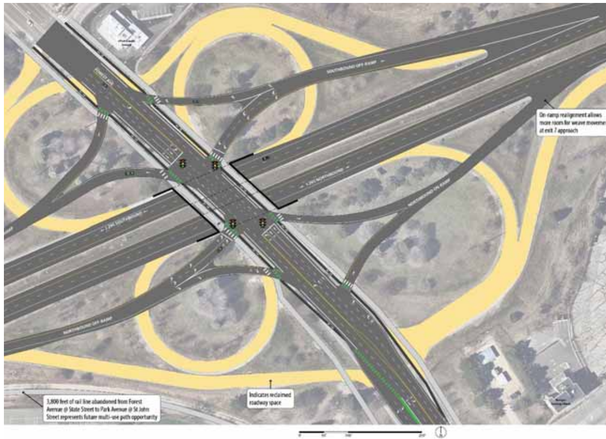
Figure 87. I-295 Exit 6 – Potential Interchange Improvement – Single Point Urban Interchange (SPUI)
