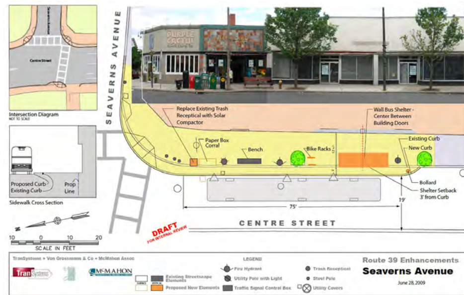
Figure 5-17: A curb extension on Route 39/Centre Street in Boston improves bus operations and provides additional space for amenities on a street with narrow sidewalks. This application could be used on Preble Street near Cumberland Avenue.
