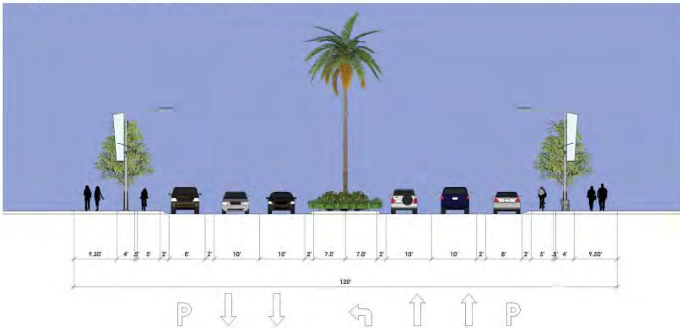
El Cajon Boulevard – Typical Section
