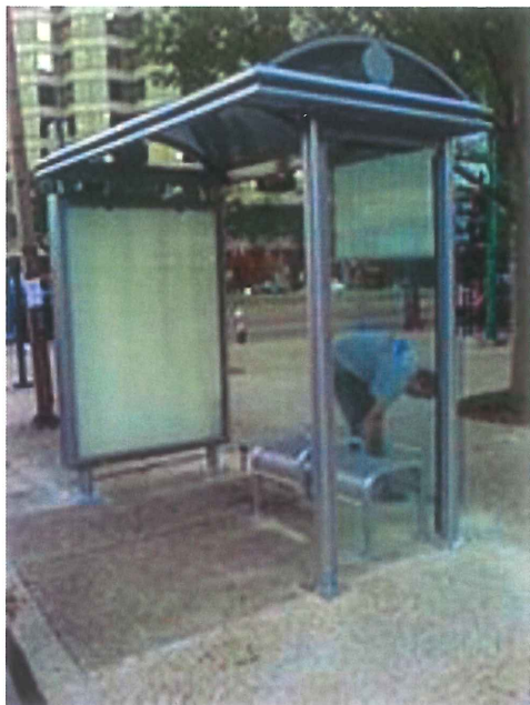
9' sierra dome roof transit shelter with bronze lexan roof panels, illuminated back-to-back advertising kiosk, 3/8" clear glass in rear and end walls, integrated map case, perforated metal bench
