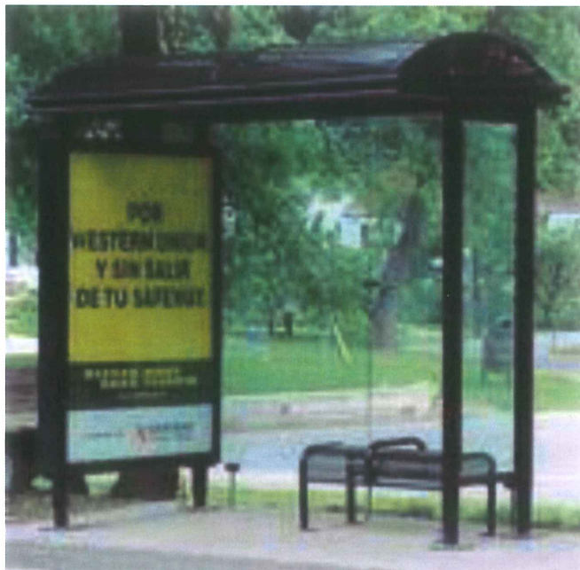
8' sierra dome roof transit shelter with a backlit flat back-to-back advertising kiosk, lexan roof panels, and 3/8" clear tempered safety glass at the back and end walls, 40" perforated metal bench with anti-vagrant bar
