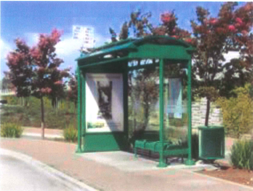
13' EURO advertising bus shelter featuring bronze lexan roof panels, Back-to-back solar illuminated Advertising KIOSK, solar led roof lighting, branded frit 3/8" glass walls, integrated map case, standard aluminum support posts with escutcheons, 6' perforated metal bench with 2 anti-vagrant bars, 26 gallon expanded metal trash receptacle
