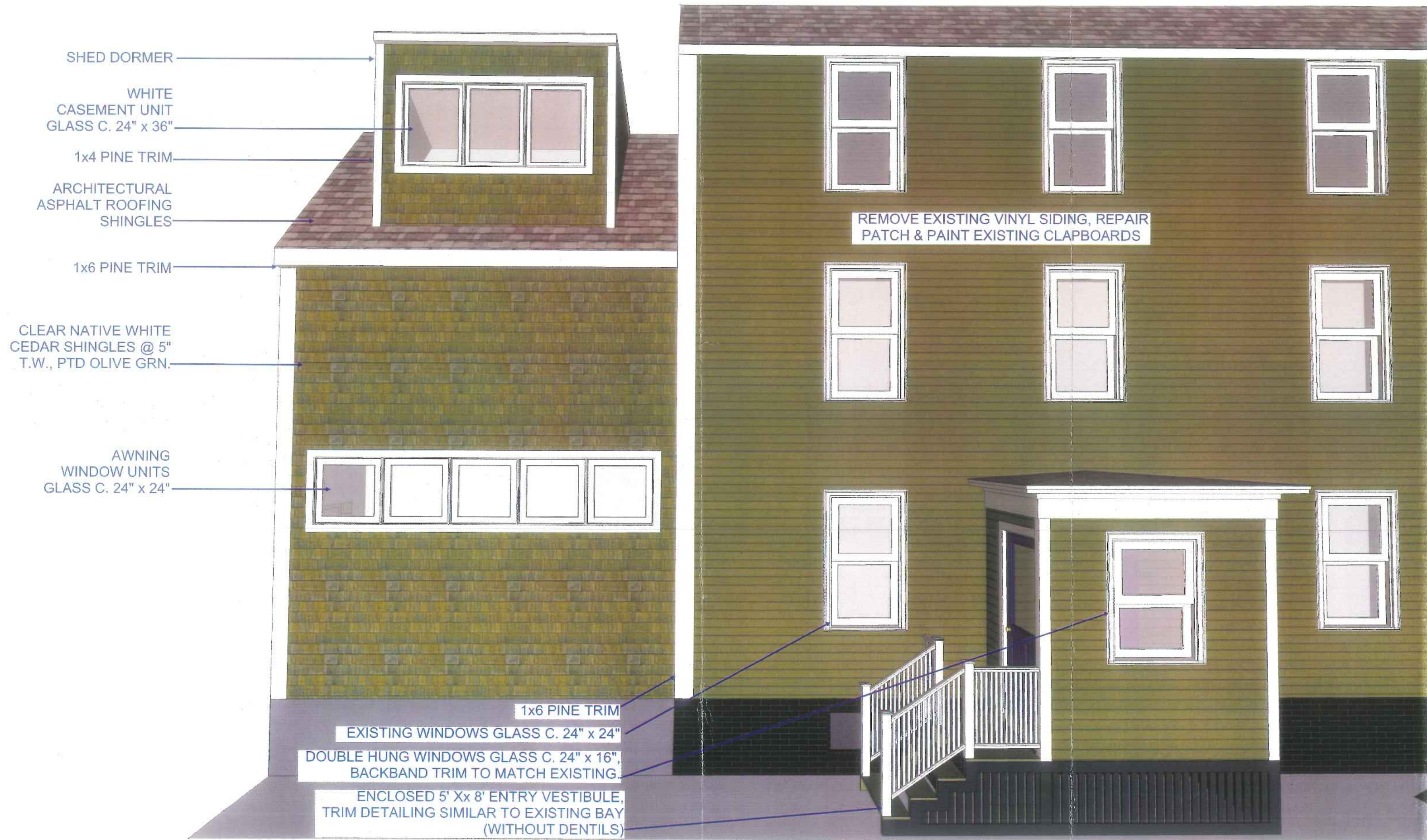
PROPOSED WEST FACADE ANNOTATED
