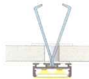
G Recessed Mounting into a Mitered Groove using a flanged Channel
