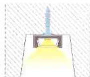
F Recessed Mounting into Mitered Groove with Bracket
