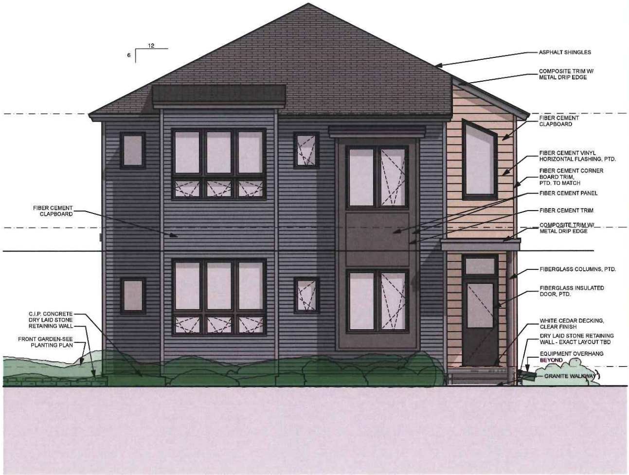
1 NORTH ELEVATION: DANFORTH ST. SCALE: 1/4" = 1'-0"
