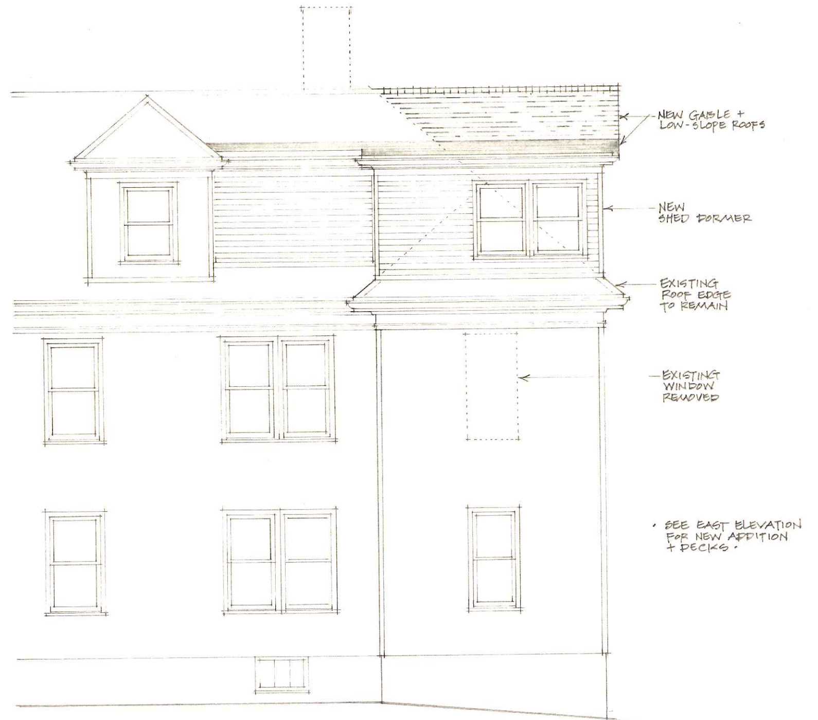
WEST ELEVATION - (PARTIAL)
