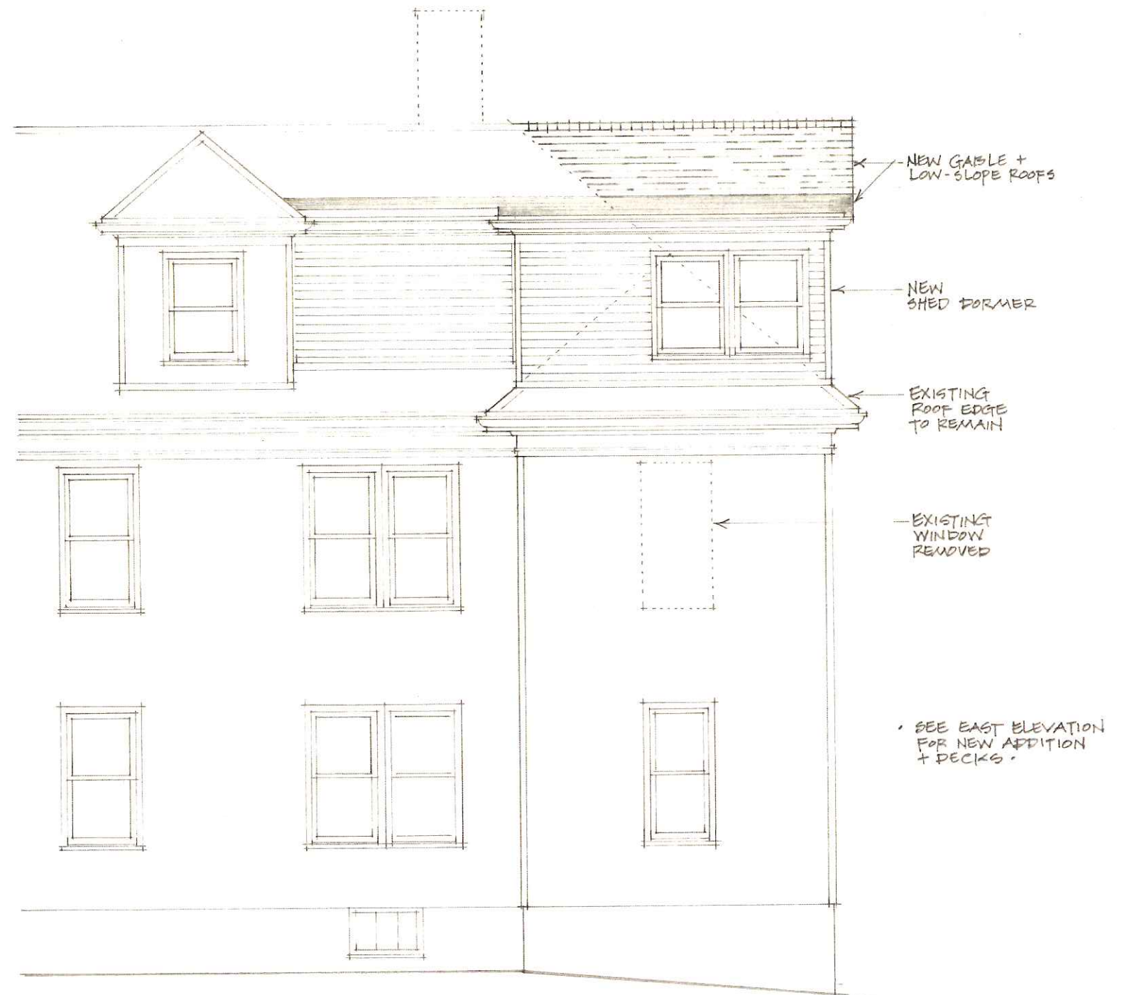
WEST ELEVATION - (PARTIAL)
