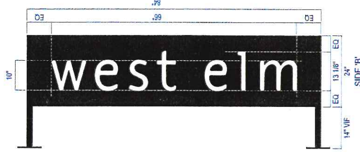
D/F ILLUMINATED BLADE SIGN | FRONT VIEW Scale: 1/2" = 1'-0"
